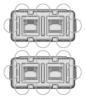
**2.** Open all 16 wing-turn latches on the front and rear of the case by lifting the latch then turning the latch counterclockwise.
